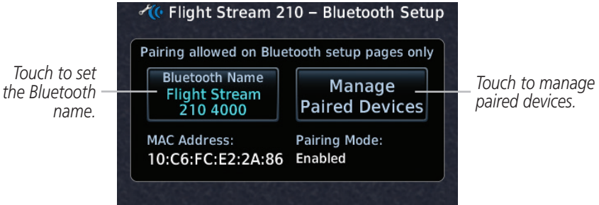
Bluetooth Setup for Flight Stream 210
