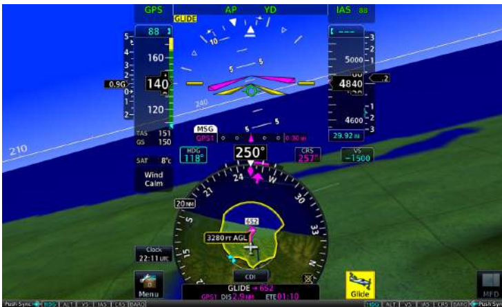
GLIDE key replaces the ADVISORY key when the status information window is not in use (full PFD only).
